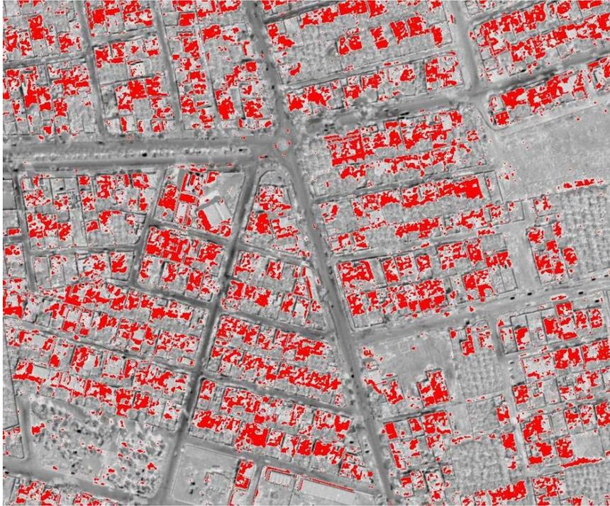
Figure 3.20: Map of damaged buildings (in red) for the Bam case study derived from a pair of Quickbird images.
